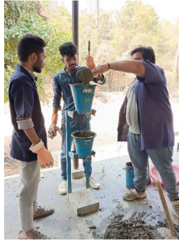
Fig: Compaction Factor Test on the Fresh Concrete
