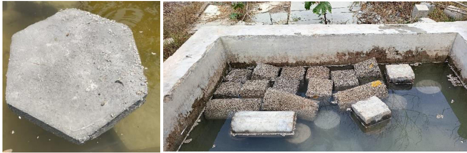
Fig: Curing of Concrete Cubes, Cylinders & Blocks
