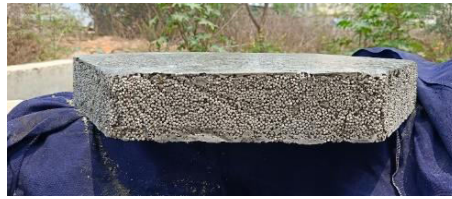
Fig: Lightweight Concrete Blocks
