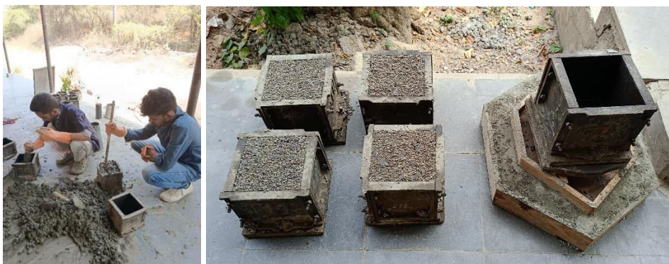
Fig: Placing and Compaction of Concrete in moulds
