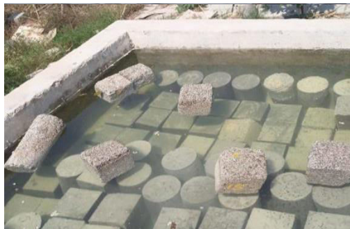
Fig 4.5: Curing the Specimens
