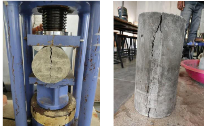
Fig 5.4: Testing of Cylinders
