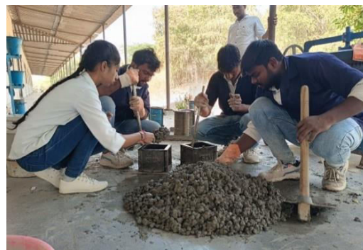
Fig 4.2: Filling the Moulds
