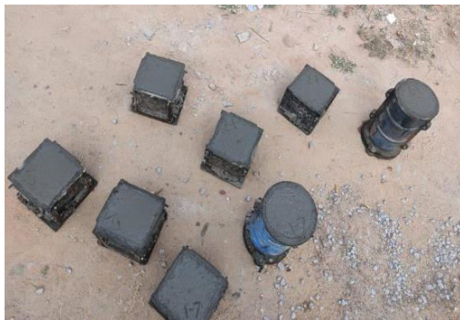
Fig 4.3: Leaving the Moulds to Dry
