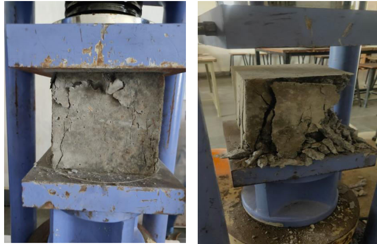
Fig 5.2: Testing of Cubes
