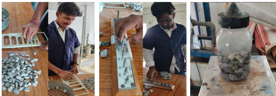
Fig 3.2: Tests on Coarse Aggregate
