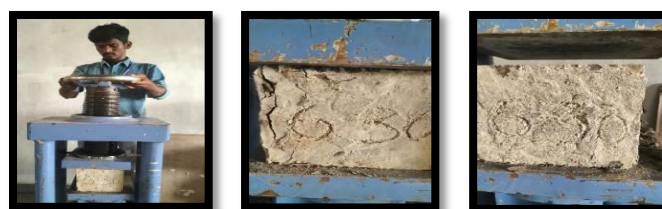
Fig – 14: Cubes of 30% replacement concrete under 28 days compression test
