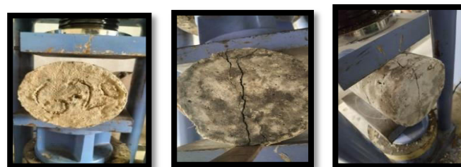
Fig – 16: Cylinders of 20% replacement under 28 day’s tensile test
