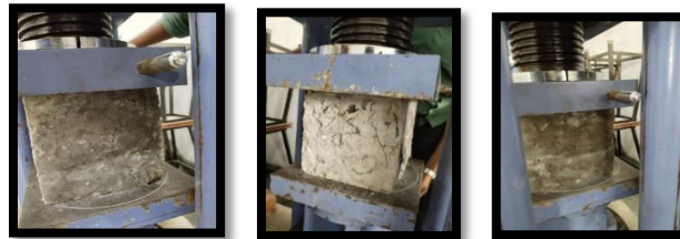
Fig- 5: Cubes of 25% replacement concrete under 7 days compression test
