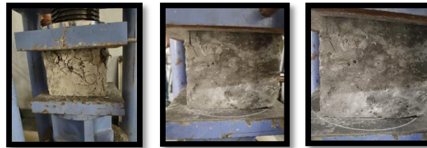
Fig – 4: Cubes of 20% replacement concrete under 7 days compression test
