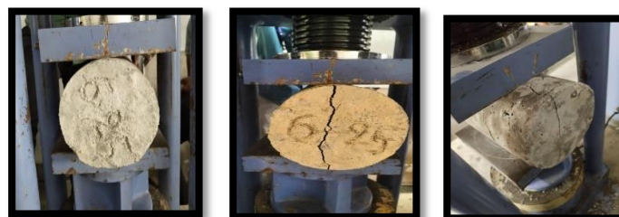
Fig -17: Cylinders of 25% replacement under 28 day’s tensile test
