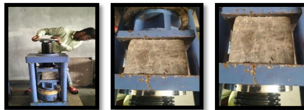
Fig -12: Cubes of 20% replacement concrete under 28 days compression test
