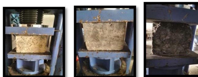
Fig-13: Cubes of 25% replacement concrete under 28 days compression test
