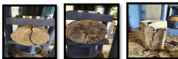
Fig – 18: Cylinders of 30% replacement under 28 day’s tensile test
