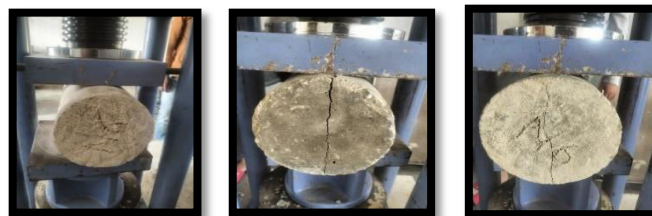
Fig –15: Cylinders of nominal concrete under 28 days tensile test
