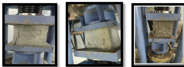
Fig – 11: Cubes of nominal concrete under 28 days compression test
