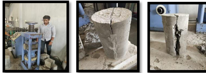
Fig – 7: Cylinders of nominal concrete under tensile test
