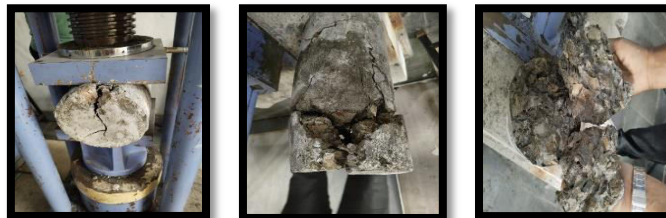
Fig -10: Cylinder of 30% replacement under 7 day's tensile test
