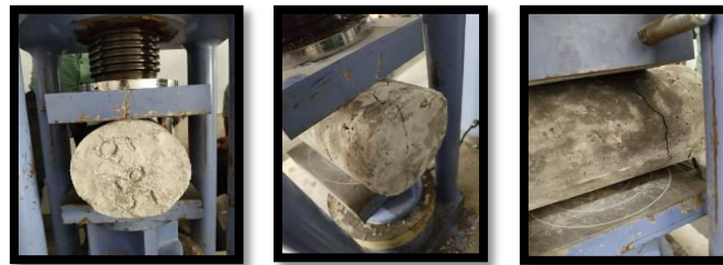
Fig- 9: Cylinders of 25% replacement under 7 days tensile test
