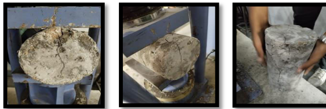
Fig –8: Cylinder of 20% replacement under 7 days tensile test
