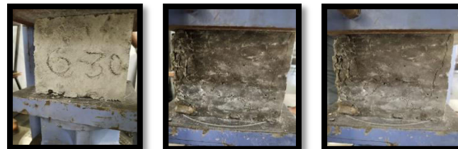
Fig – 6: Cubes of 30% replacement concrete under 7 days compression test
