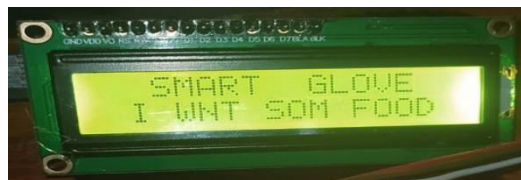
Fig 6 :-Lcd display shows the user inner needs when they move their fingers and also voice play back in speaker
