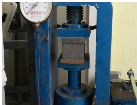
Figure 8 : Testing of 10%MSW specimen at 7 days curing
