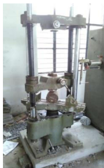
Figure 9: Split tensile strength testing at 14 days curing
