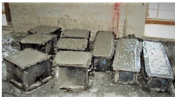
Figure 6: casting of samples (cubes and prisms)
