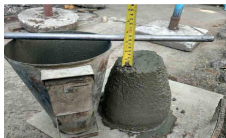
Slump cone test
