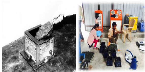
Filling the mould (for 150 mm cube 3 equal layers)
