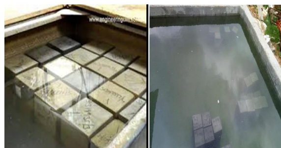
Curing of cubes and cylinders
