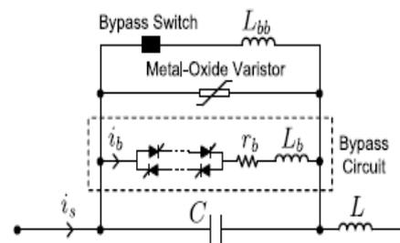
Fig-1. Design of a single phase RFCL.
