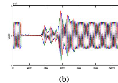
Fig.7. Responses of the nine-bus system subsequent to the strike of fault  $Flt_A$ . (a) Line currents. (b) Capacitor voltages.
