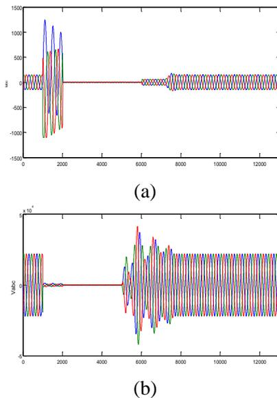
Fig.8. Responses of the nine-bus system subsequent to the strike of fault Flt<sub>b</sub>.(a) Line currents. (b) Capacitor voltages.
