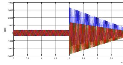
Fig. 5. Instantaneous currents through breaker CB5 in the nine-bus system (left column) and its equivalent network (right column) with the RFCL in line L45.
