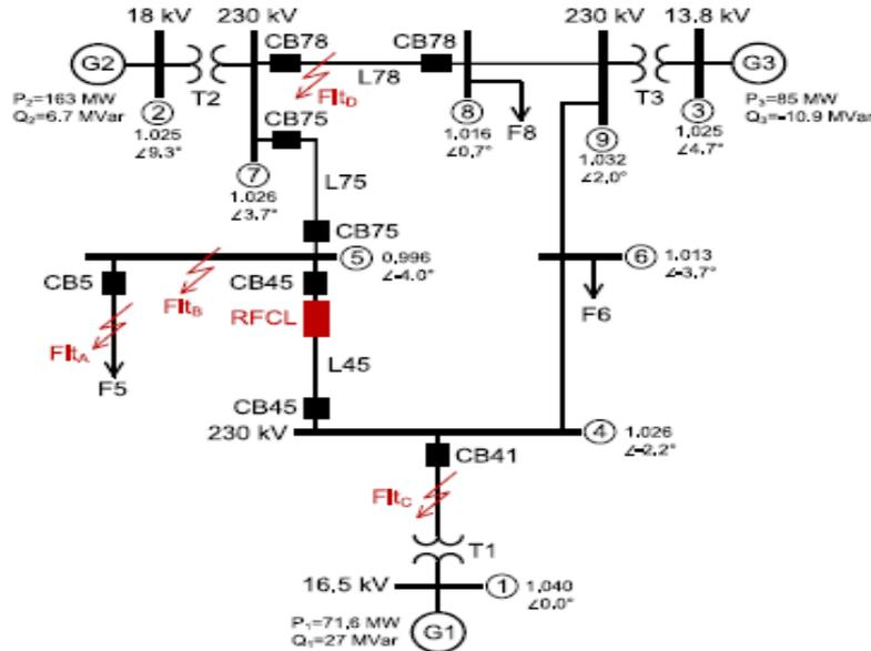
Fig. 2. Test power system with an RFCL inserted between bus 5 and 4.
