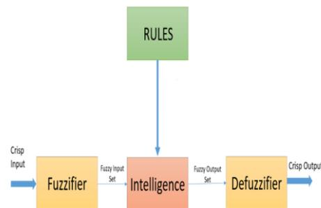
Fig.5 Schematic diagram of fuzzy.
