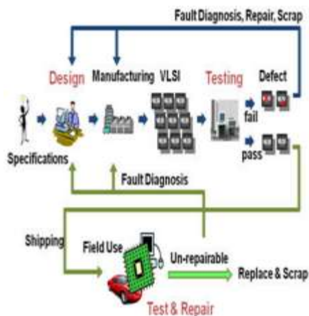
Figure 1 : VLSI realization process
