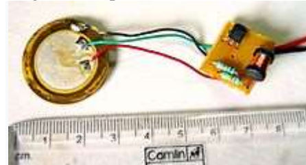
Interior of a readymade loudspeaker, showing a piezoelectric-disk-beeper (With 3 electrodes ... including 1 feedback-electrode ( the central, small electrode joined with red wire in this photo), and an oscillator to self-drive the buzzer.
