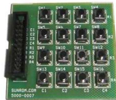
Figure: matrix keypad on PCB board.
