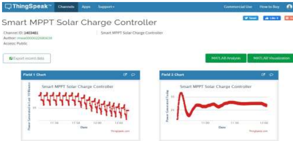
Fig. 8. Generated Power Data Available on Thingspeak (IoT)
