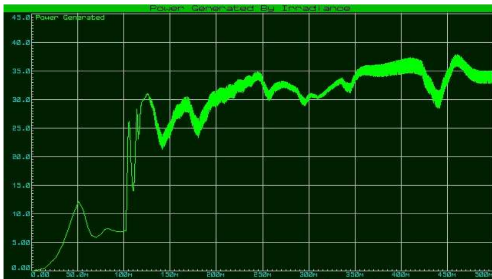
Fig. 9 Graph Analysis of the power generated by Smart MPPT using P&O MPPT at Stable irradiance conditions.
