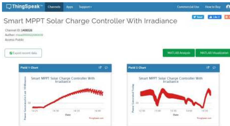
Fig. 9 Graph Analysis of the power generated by Smart MPPT using P&O MPPT at Stable irradiance conditions.
