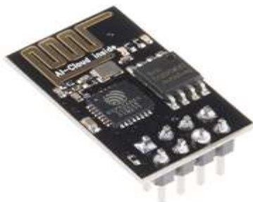
Figure 4. ESP8266 ESP-01 module / ©Sparkfun
