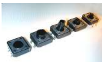
Figure:4. switches in a row
