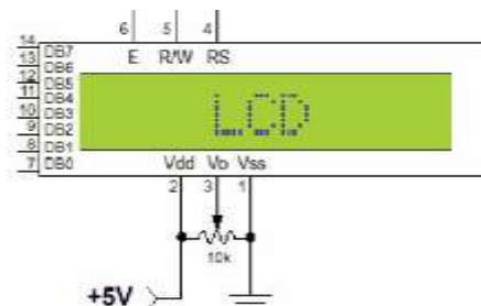
**Figure.2. Pin diagram of 1x16 lines LCD**
