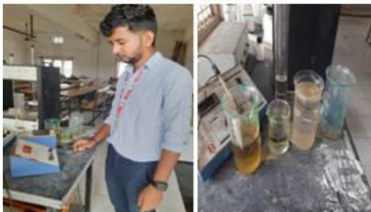
Figure 5 Turbidity test and Water samples
