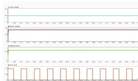
Fig 6. Simulation results of buck converter
