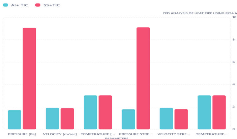
Figure 30: Validation of Heat pipe fluid R214 a with different materials
