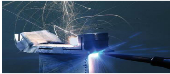
Fig 6: Turbine blade during laser drilling
