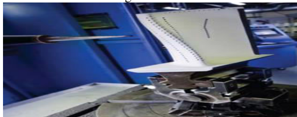
Fig 7: Laser drilling turbine blade
