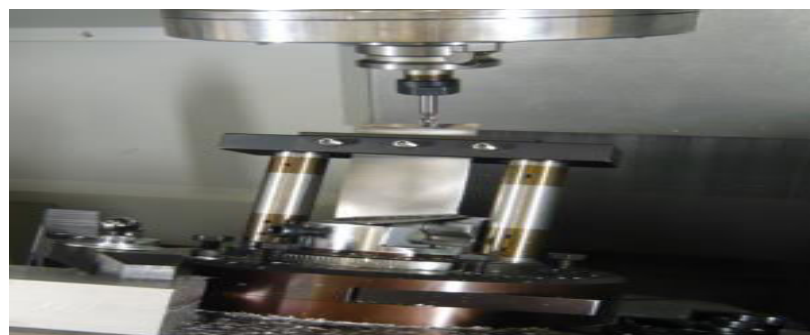
Fig 9: Adaptive CNC blending of repaired air foil tip
