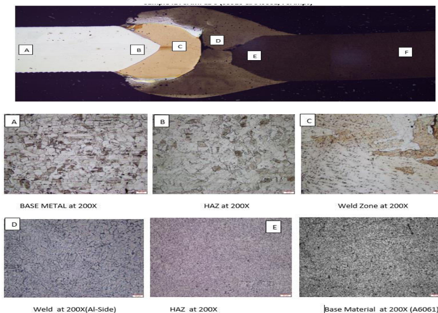
Figure 13: Sample-2 micro structure with different specimens in 60 Amps
