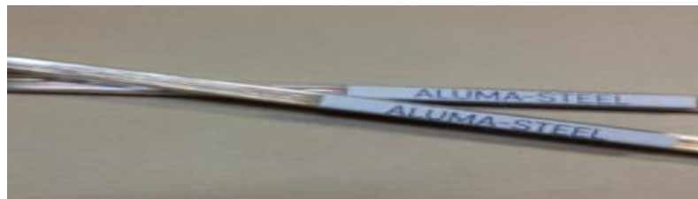
Figure 2: showing welding rod- filler rod
