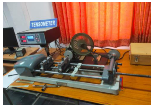
Figure 9 Electronic tensometer for tensile & flexural testing
