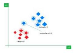
Now, given another set of data points (also called testing data), allocate these points to a group by analyzing the training set. Note that the unclassified points are marked as 'White'.
