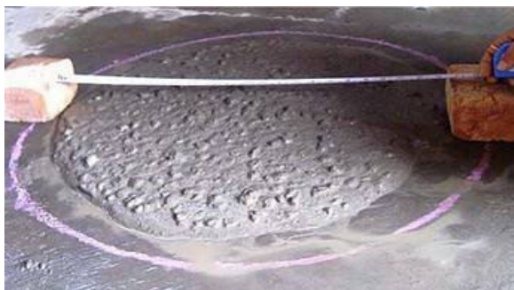
Slump flow test
