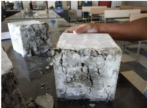
Specimen tested after acid attack
