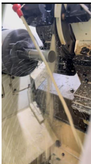
Figure 2 Wet cooling condition
