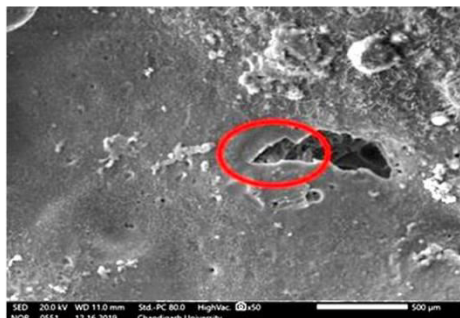
Fig 18: SEM image of EDM cut sample at 20% SiC showing sharp edged voids
