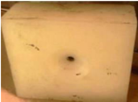
Fig 7: Nylon Fixture for holding the work piece
