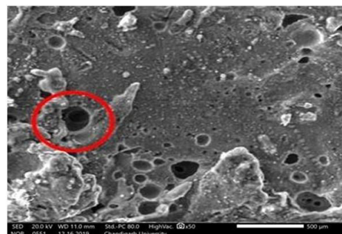
Fig 17: SEM image of EDM cut sample at 30% SiC showing rounded pore features
