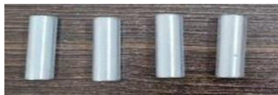
Fig 6: Some specimens obtained after stir casting process
